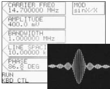
Exact bandwidth of the \sin x/x modulated burst is menu-selectable.
